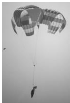
Fig. 4: Cross parachutes for deceleration and stabilization
