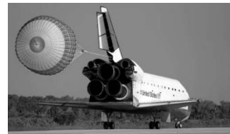
Fig. 5: Hemisflo parachute for space probe, capsule or module and shuttle deceleration
