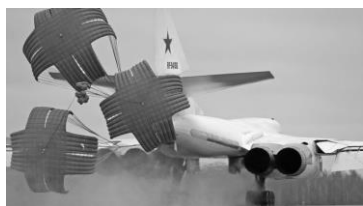
Fig. 4: Cross parachutes for deceleration and stabilization
